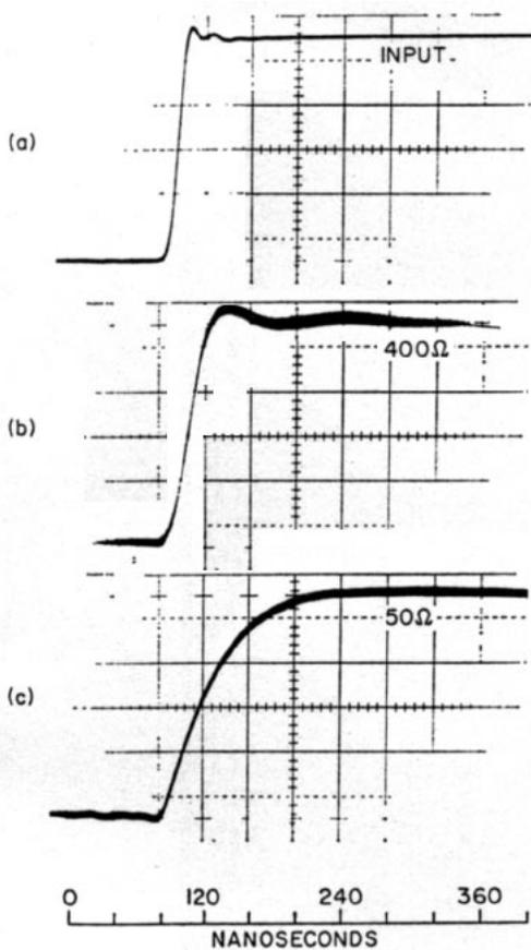
Fig. 3. An input magnetic field test waveform (a), and the relative responses of 1 m<sup>2</sup> antenna systems. The output of a 400Ω system with differential follower is shown in (b), and the output of a 50Ω cable system in (c).
