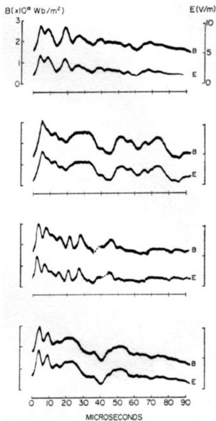
Fig. 4. Correlated magnetic (*B*) and electric (*E*) field waveforms from lightning at a distance of 50-100 km. The same vertical scales apply to all records.
