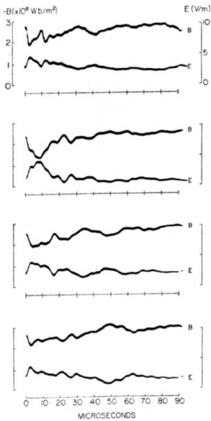
Fig. 5. Correlated magnetic ( $B$ ) and electric ( $E$ ) field waveforms from lightning at a distance of 50-100 km. The magnetic fields are inverted with respect to the electric because  $\phi$  in Eq. (1) was close to  $\pi$ .
