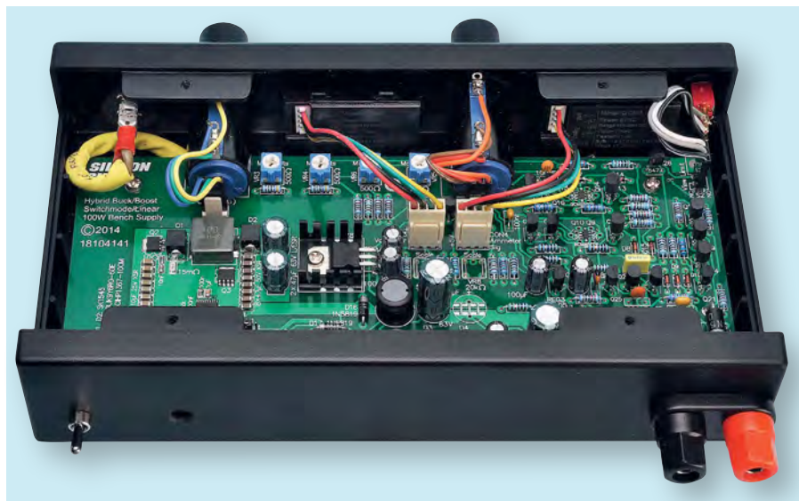
Another view inside the case, this time from the rear. The rear panel carries the power switch (S1), a hole to access the DC socket and the two output terminals (note: prototype PCB shown).
